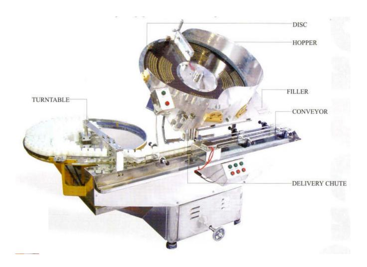
This model is equipped with sophisticated technology and superior production techniques in order to get higher production in counting and filling of capsules / tablets. Up to 4 bottles can be automatically filled at a time through a twin 4 track filler. Maximum output of 100 bottles / minute depending upon the number of counts per fill.
